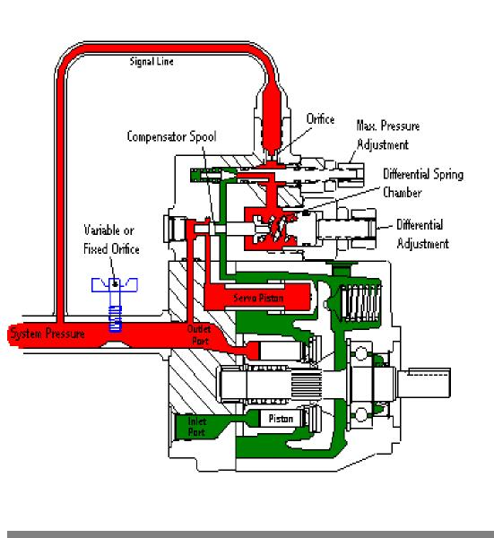
Increasing the pump drive speed will increase the pump output flow, but since the load sense control is working to maintain a constant pressure drop across the orifice, the load sense pump will destroke to maintain the same output flow.
