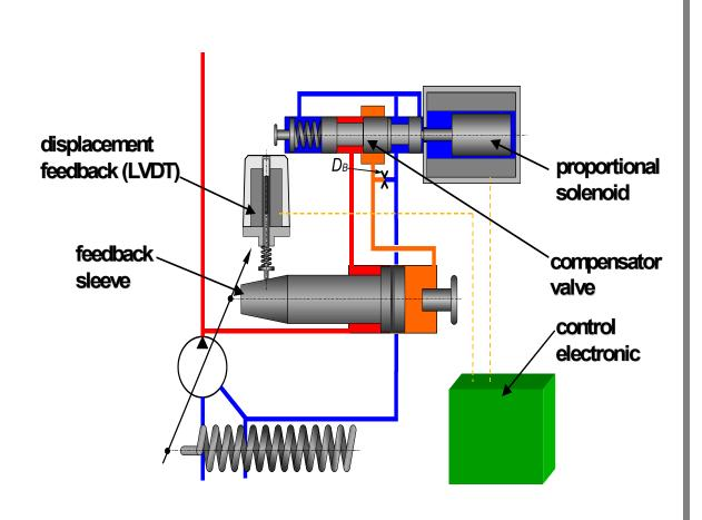
A proportional displacement control will position the swashplate angle proportional to a input voltage signal to the solenoid. The output flow can be adjusted, without affect from system pressure. A LVDT feedback signal of the swashplate angle closes the loop electronically. An amplifier card in the electronic controller compares the command signal and the feedback signal and sends a voltage signal to the proportional solenoid to position the swashplate.
