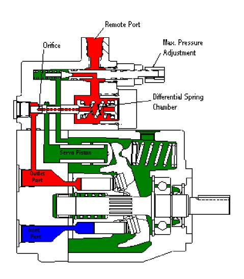
Just like a standard Pressure Compensator, except the pressure limiter adjustment is done with an external relief valve.
