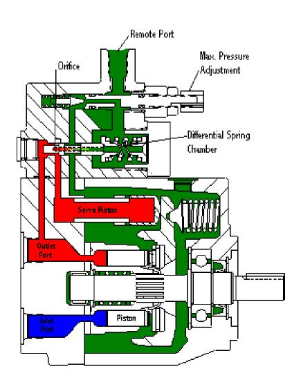
As Pump Pressure reaches setting of remote relief valve, the pressure in the differential spring chamber is limited and the spool shifts to destroke the pump.
