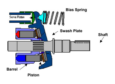
Outlet Flow can be varied by changing the shaft drive speed, or by changing the swash plate angle
