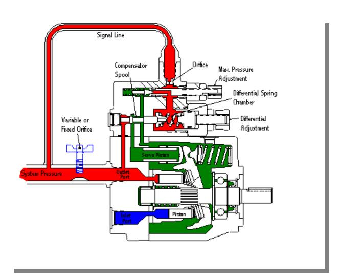
In this view the variable orifice is wide open and it is not restricting the pump flow. Pump outlet pressure and load pressure are equal. Since the pressure is equal on both sides of the spool, the differential spring keeps the spool to the left. There is no control pressure in the servo piston, so the pump will stay at full stroke.
