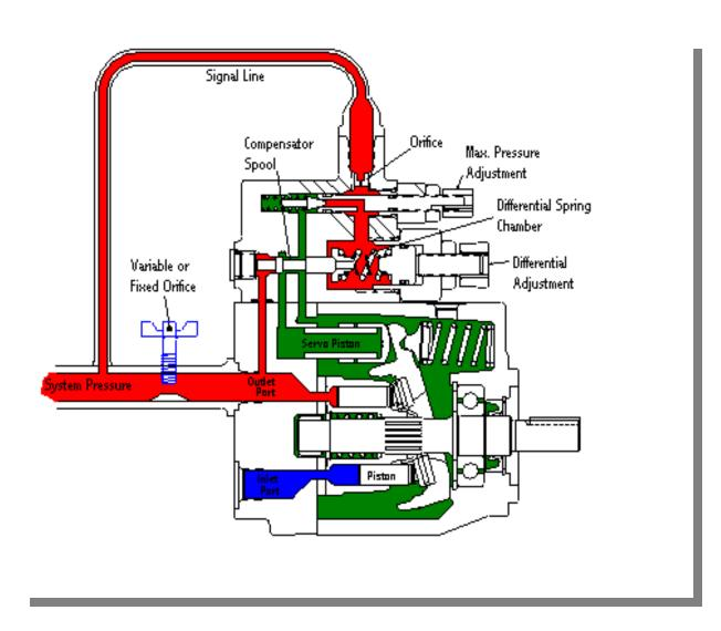
A load sense compensator will react to increases in the load by increasing output pressure. This is done by sensing the pressure drop across an external orifice and adjusting displacement to maintain a constant pressure drop across the orifice.
