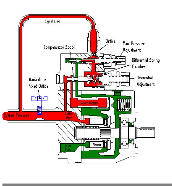
In this view the variable orifice is restricting pump flow. Pump outlet pressure is increased and a pressure drop is created across the orifice. The pump pressure will increase until it overcomes the differential spring force and shifts the spool to direct control oil into the servo piston and destroke the pump. The pump will maintain a flow level that keeps the pressure drop across the variable orifice constant ( equivalent to the differential spring setting).
