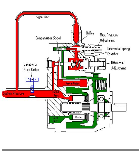
Since the load sense control will adjust pump flow to maintain the pressure drop across the orifice constant, increasing the orifice size will increase the flow to the system. Closing the orifice, will decrease the flow to the system.
