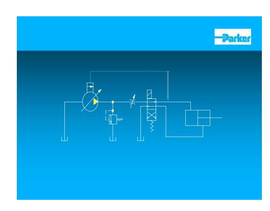
Remember the Pressure Compensator system used 8.7 HP and wasted 2.9 HP
