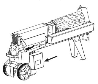
This Log Splitter is equipped with a ZHB Control System that requires it to be operated with both hands (the left hand controls the Hydraulic Control Lever while right hand controls the Pushbutton Switch). The Log Splitter will freeze when either hand is absent. Only after both hands release the controls, will the Log Pusher return to the starting position. **AWARNING:** Never force the Log Splitter for more than 5 seconds.
