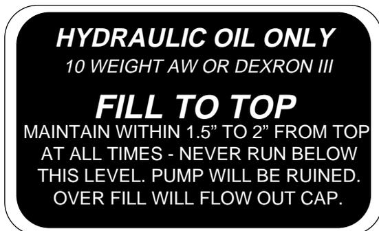
**NOTE:** There are two reservoir tank capacities depending on the log splitter model. The large tank has a capacity of approximately 7 gallons. The small tank has a capacity of approximately 4 gallons.
